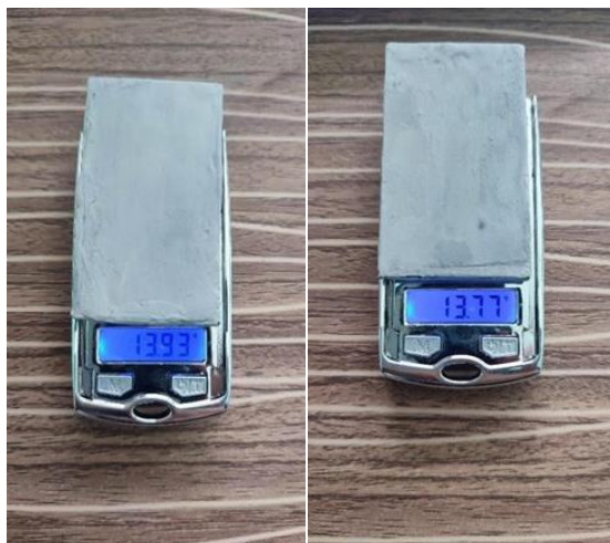
Figure 33 and 34. Weight of Sample C (left) and Sample D (right) after 15 minutes of immersion to Hydrochloric Acid.
