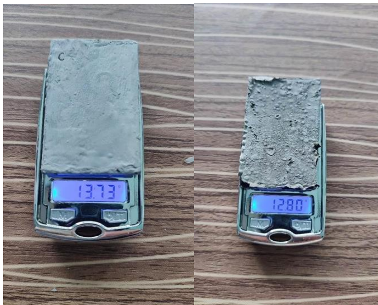
Figure 38 and 39. Weight of Sample C (left) and Sample D (right) after 30 minutes of immersion to Hydrochloric Acid.
