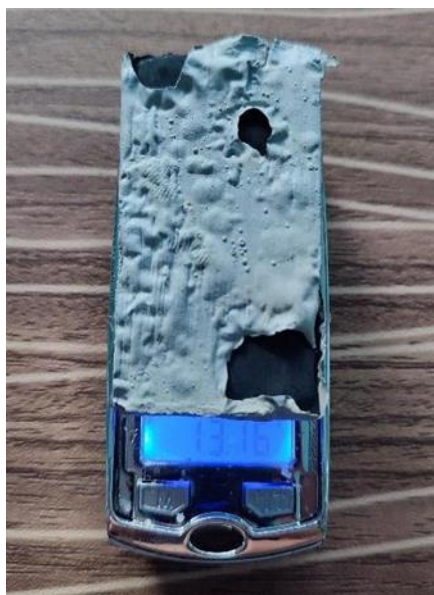
Figure 43 and 44. Weight of Sample C (left) and Sample D (right) after 45 minutes of immersion to Hydrochloric Acid.
