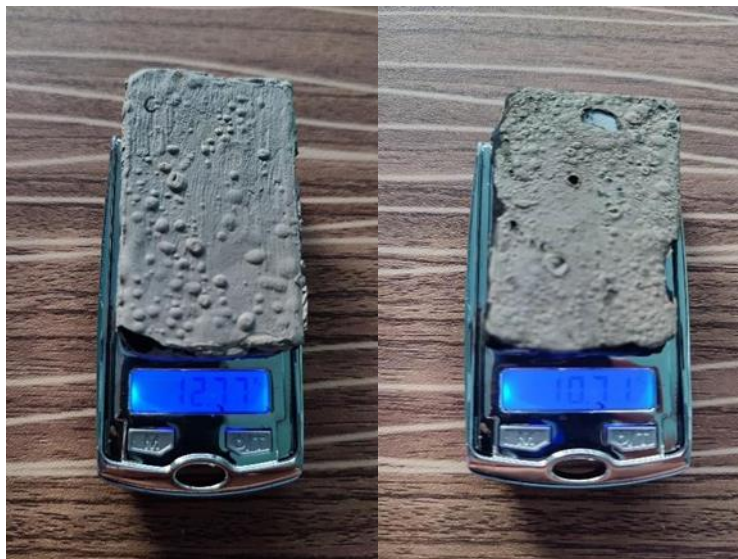
Figure 43 and 44. Weight of Sample C (left) and Sample D (right) after 45 minutes of immersion to Hydrochloric Acid.
