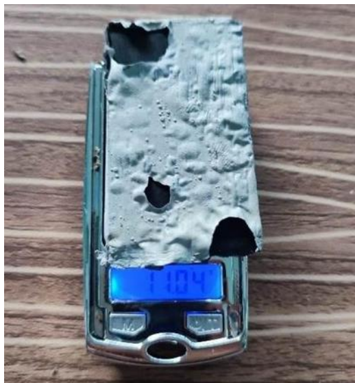
Figure 50. Weight of Plain sample after 60 minutes of immersion to Hydrochloric Acid.
