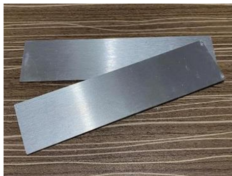
Figure 4. 6061 Aluminum Alloy Sheet Metal (20x5x.02cm)
