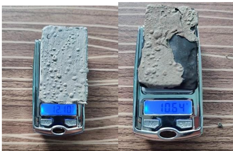
Figure 48 and 49. Weight of Sample C (left) and Sample D (right) after 60 minutes of immersion to Hydrochloric Acid.
