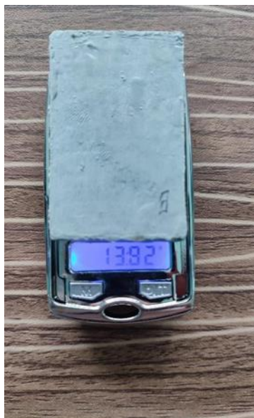
Figure 35. Weight of Plain sample after 15 minutes of immersion to Hydrochloric Acid.
