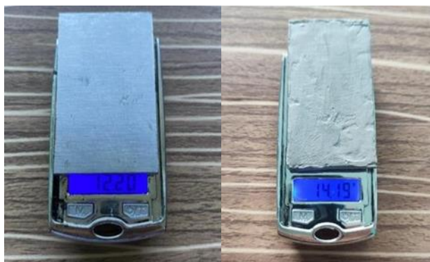
Figure 26 and 27. Initial weight of Bare metal (left) and Sample B (right) before immersion to Hydrochloric Acid.
