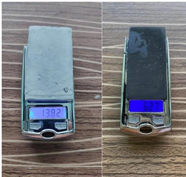
Figure 36 and 37. Weight of Bare metal (left) and Sample B (right) after 30 minutes of immersion to Hydrochloric Acid.
