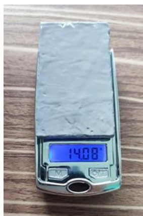
Figure 30. Initial weight of Plain sample before immersion to Hydrochloric Acid.
