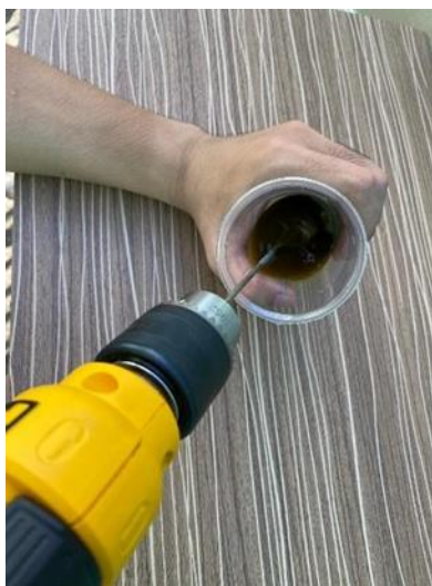
Figure 14. Mixing the Mango Leaf extract to the Epoxy Primer
