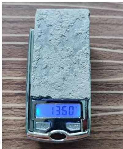
Figure 40. Weight of Plain sample after 30 minutes of immersion to Hydrochloric Acid.
