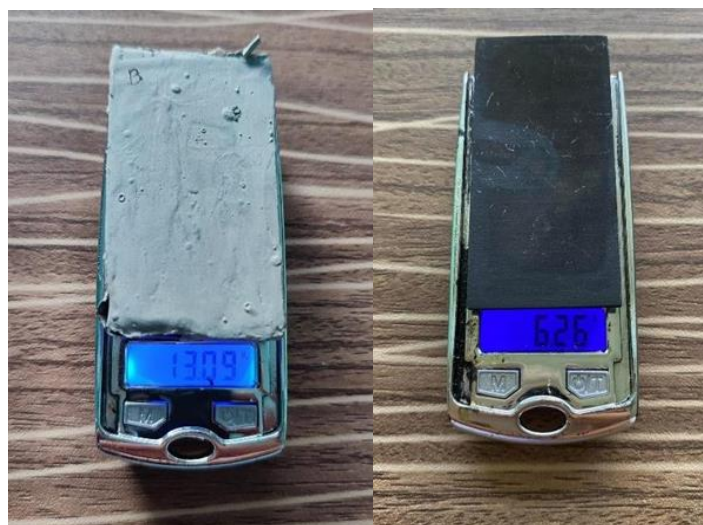
Figure 41 and 42. Weight of Bare metal (left) and Sample B (right) after 45 minutes of immersion to Hydrochloric Acid.
