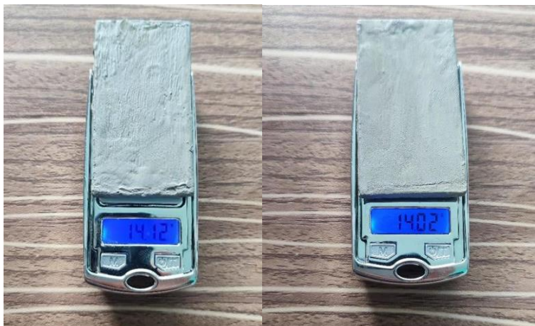
Figure 28 and 29. Initial weight of Sample C metal (left) and Sample D (right) before immersion to Hydrochloric Acid.
