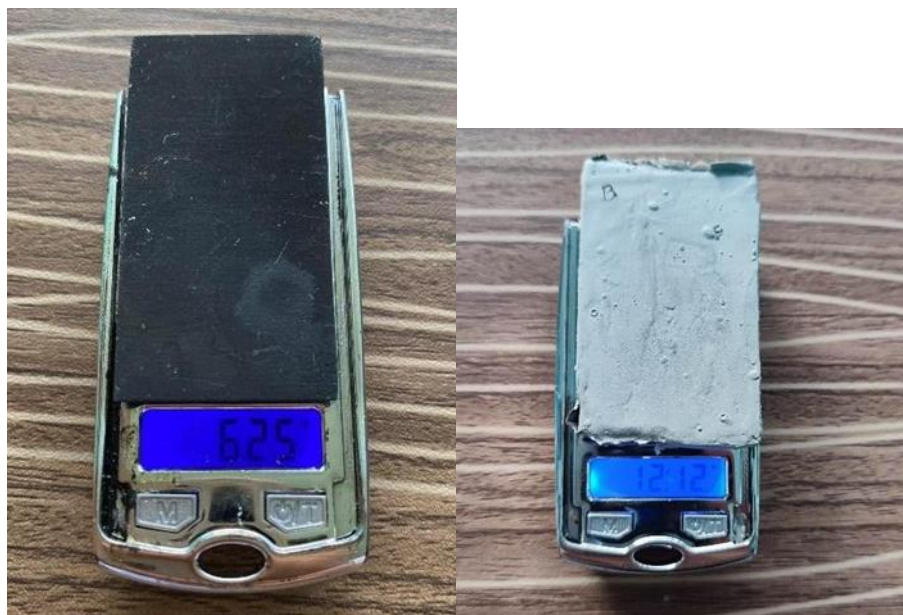
Figure 46 and 47. Weight of Bare metal (left) and Sample B (right) after 60 minutes of immersion to Hydrochloric Acid.
